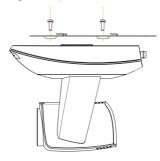
5. Push forward camera's bottom slide according to the mounting plate's bottom slide until they reach their limit. Fix the ceiling mount plate and camera's bottom plate with M3x8 screws.
